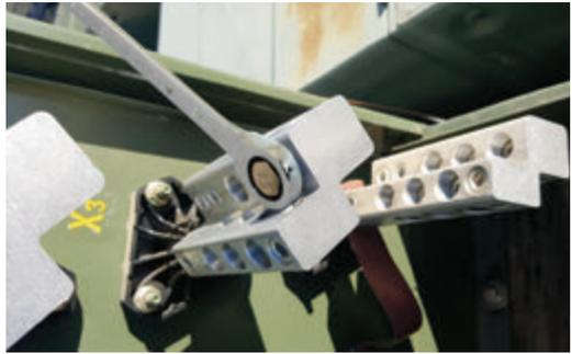
The low profile design allows access to connectors when space is limited. Just 1/2" is exposed above the bar, while a 1/2" allen driver fully engages the connector to avoid stripping. Low profile means less chance of touching other connections or exposed metal.
