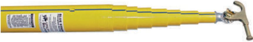
The BLUE STRIPE® Heavy Duty Telescopic Stick has been designed for maximum strength. The wall thickness of section #1 is nearly double that of a standard foam filled section. The machined spline end assembly is pinned and glued to handle higher torque applications.
