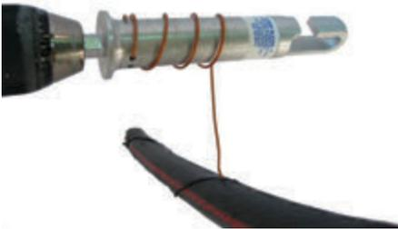
The Strip-N-Coil uses small holes at the base to hold a single concentric neutral wire. Twisting along the cable easily cuts
