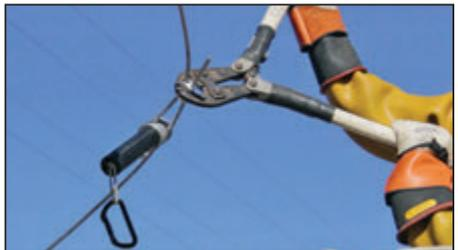
3. The Double Sided Clamp **holds two conductors simultaneously**. Easily attach parallel groove and crimp connectors.
