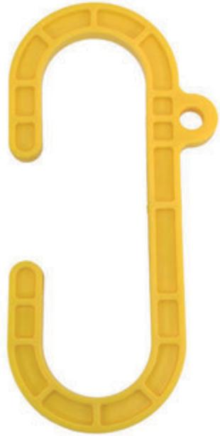
Multiple Jumper Hooks effectively support and cradle long stretches of jumpers. The Jumper Hook installs easily with a gloved hand or shotgun stick. They will fit over any class 2 or 3 line hose and exhibits a flash-over resistance of over 50 kV.
