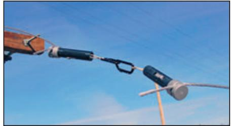
2. **Safely cut slack conductors** (up to 200 lbs. of tension between Clamp & Carabiner) while maintaining positive control of loose ends.
