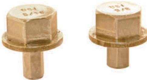
The Padmount Hex Adapter Set includes two 3/4" drivers for a 3/8" and 5/16" Allen head connector commonly used on busbars inside URD pad gear. Works with any 3/4" open-end or box-end wrenches and any type of socket drivers (ratcheting or powered).
