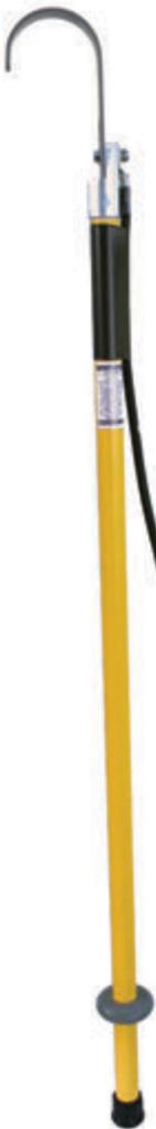
The Utility Solutions BLUE STRIPE® Discharge Hook safely eliminates a static charge after de-energizing. It is a 1¼” diameter, 4’ straight stick made of high performance closed cell foam and includes a tin plated copper “U” hook and 6’ of copper grounding cable attached to a 2” aluminum “C” type clamp with serrated jaw.
